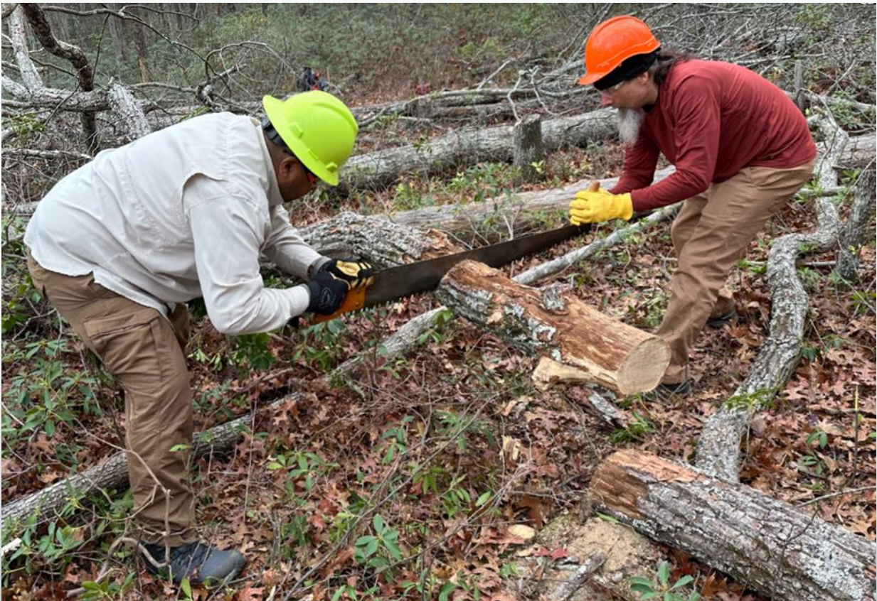
Luis Betancourt and Rich Seriani lean into a 2-man crosscut saw. Note proper PPE usage.
